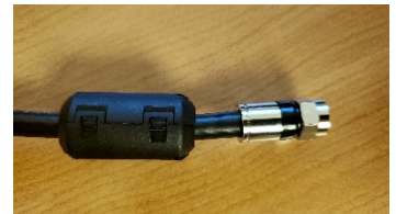
Figure 10 - Ferrite Choke installed on RG6 Coax cable
