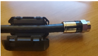
Figure 9 - RG6 Coax cable laying in Ferrite Choke
